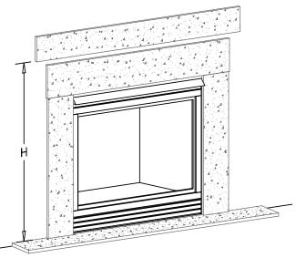
The Portico Mantel's design allows viewing straight through to the wall. An additional (57x6) marble/granite piece can be installed to carry the natural stone theme throughout the surround. The additional piece will need to be installed **BEFORE** the mantel is attached to the wall.
