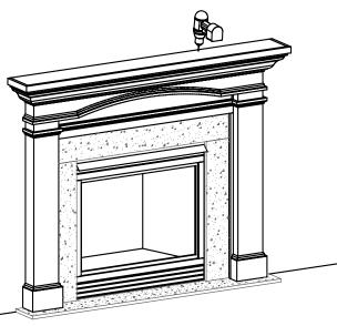
Center and place mantel on wall overlapping the noncombustible facing material with the top resting on the ledger strip. Using an electric drill, predrill 1/16" holes down through the top into the ledger strip. The holes should be drilled 1" off of the back edge of the top. Attach the mantel to the ledger board using (3) 4D finishing nails (provided) through predrilled holes. Use a nail set to set the nail head below surface of mantel, and fill the resulting hole with an appropriate filler.
