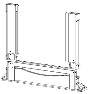
Position the top assembly (a) of mantel upside down on a flat, clean, non-abrasive surface. If scribe molding (d) was shipped attached to the leg and breast board, remove it before beginning assembly. Pry gently from the rear with a flat screwdriver.
