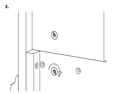
Push down on the leg until dowels are fully inserted into the breastboard and there is no gap between leg and breastboard. Using a philips screwdriver, turn the cams in breastboard clockwise until snug. Do not rely on the cam to pull the two together. **Do not over-tighten**, as too much torque can break the cam. Repeat the last two steps for the other leg.
