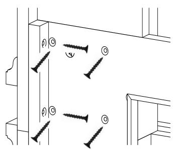
Additional strength can be added to the assembly by inserting (8) 1.25" drywall screws through the predrilled holes on the breast board and (4) 1.25" drywall screws through the side returns, Make sure the seams and edges are tight and square.
