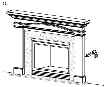
Caulk the mantel to the wall all the way around, using a caulk that matches your mantel color. This will eliminate any remaining gap between mantel and wall.
