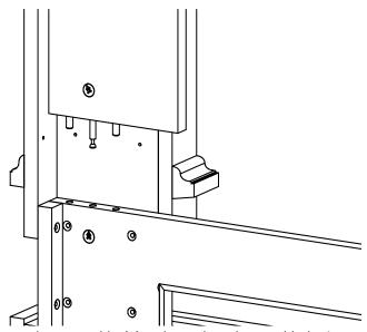
Attach one leg assembly (c) to breastboard assembly by inserting dowels and cam pin into matching holes on ends of breastboard. Before inserting, make sure that the arrow on the cam in breastboard points toward the edge of board as shown in inset. (Dowels and cam pins are shipped pre-inserted in the end of the leg assembly.)
