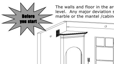
The walls and floor in the area of the installation should be clean, plumb and level. Any major deviation should be remedied before installing the fireplace, marble or the mantel /cabinet.
