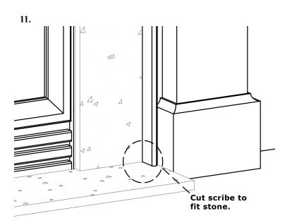
If using a hearth that fits between the leg opening, cut the scribe to allow for stone height between the legs. Place the scribe molding as shown above, positioning it so that it just contacts the noncombustible surround. Be careful not to hit the facing material when nailing the scribe in place. No cutting is needed if hearth exceeds mantel legs.
