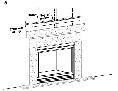
Measuring down from the first line the thickness of the mantel top, mark two points and draw a second line. This line positions the top of the ledger board.
